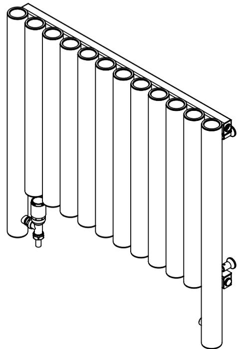
We recommend the 3 Bar Safety Valve for all ELECTRIC ONLY (E) products. Dual Fuel is possible either by use of "T" piece and radiator valve or by use of ONE850 or ONE851 (4 way valve)
