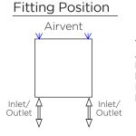
Vertical Mount All Dimensions are in mm Max.Working Pressure = 10 Bar Max.Working Temperature = 95° Inlet/Outlet: 1/2" BSP Fuel: E/H/D
