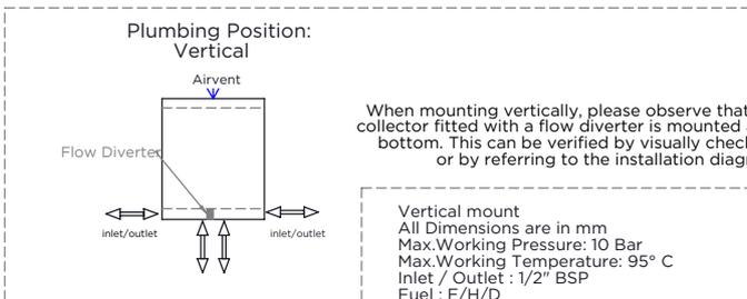
When mounting vertically, please observe that the collector fitted with a flow diverter is mounted at the bottom. This can be verified by visually checking or by referring to the installation diagram
